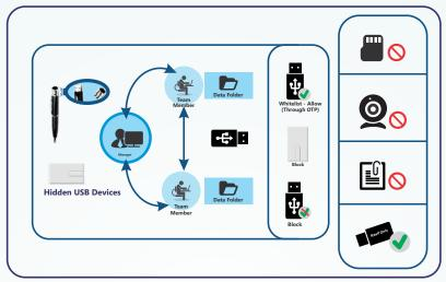
eScan Enterprise DLP's advanced Device Control feature helps in monitoring USB devices that are connected to the endpoints in the network. On Windows endpoints, administrators can allow or block access to USB devices such as webcams, CD-ROMs, composite devices, smart-phones, Bluetooth devices, SD cards, or imaging devices. Unauthorized access to external devices can be blocked using password protection, thus preventing data leakage through USB devices
